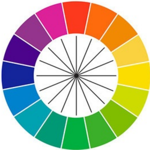
Figure 10.9 The Color Circle. Colors opposite each other are complementary; that is, equal amounts of light in those colors cancel each other out, producing a neutral gray.
